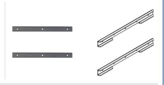
This adapter allows you to convert the hole pattern of your LCD TV mount. It converts hole patterns from VESA 100x100 to 100x200. Ideal to mount larger LCD/TFT monitors to wall-, desk- and ceiling mounts.
