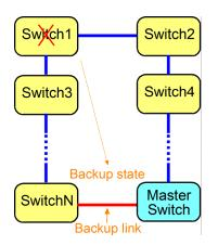
The redundant ring function can support not only one fault case but also multiple faults cases at the same time and give much faster reponse time than typical Spanning Tree Protocol.
