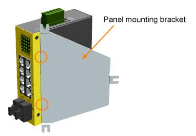
2. Screw the bracket on the switch unit.
