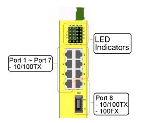
**Model 800M-2 series** provide eight 10/100TX copper ports and two 100FX fiber connectors. Port 7 and Port 8 support dual network cable types.
