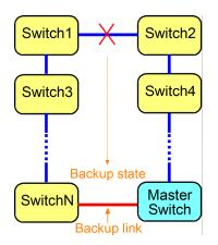
From standby state, the backup link enters into backup state. Other faults could be a switch failed due to function failure or power problem as shown below:
