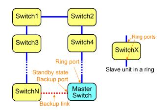
Slave Units: All switch units except the master switch in a ring configuration
