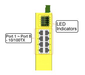
**Model 800M-1 series** provide eight 10/100TX copper ports and one 100FX fiber connector. Port 8 supports dual network cable types.
