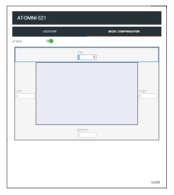
**NOTE:** If wanting to adjust the bezel in a format other than pixel, return to the device view within the device list from configuration and open the HDMI OUTPUT tab. Scroll to the under the Video Wall slider and select the unit type for adjustment (Pixels, Millimeters, or Inches). Select Bezel Compensation from the Edge Compensation drop down and then enter the correct amount, before pressing the save button.
