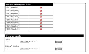
HDBaseT Receivers Link status - A red circle will display when no receiver is connected or it is receiving no signal. A green circle will display when there is a receiver connected.
