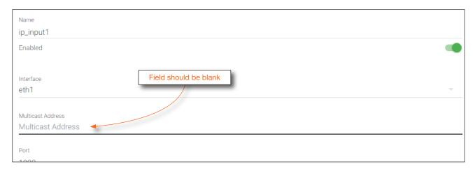
9. Unicast setup is complete. The decoder unit will now receive streams exclusively from the encoder containing the IP address of this decoder.
