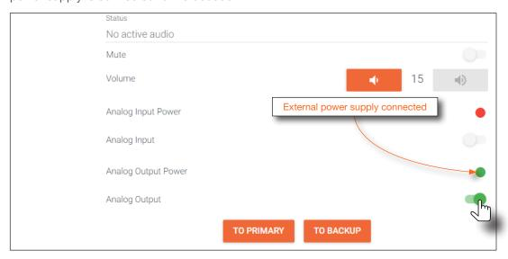
8. Audio from the source will now be heard on the **ANALOG OUT** port of the decoder. Note that when audio is deembedded, it will not longer be audible using the HDMI OUT port on the decoder.
