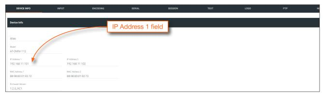
9. Locate and make note of the IP address of the encoder, which can be found in the **IP Address** field. If using dual-channel encoders, use the IP address in the **IP Address 1** field.
