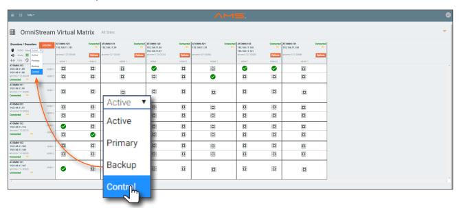
6. The Control screen will be displayed. In the Control screen, **HDMI** ports are replaced with control ports: **Port 1** In / Port 1 In for encoders and **Port 1 Out** / **Port 2 Out** for decoders.
