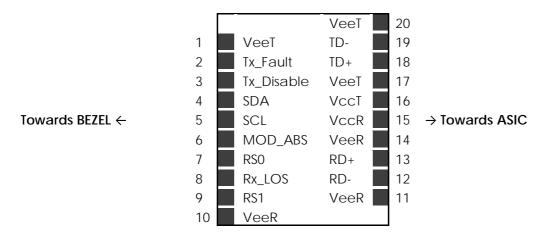
Figure 2. Transceiver Electrical Pad Layout
