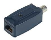
IP01 is a low cost and easy, speedy solution to allow you use existing coax cable to send IP camera signal. Used in pairs with your RG59 cable to exceed the IEEE 802.3 10BaseT NEXT specification. The working range could up to 200 meters at 10Mbps speed.
