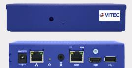
4K UHD IPTV End-Point which delivers interactive viewing portals and advanced network video decoding. Its fanless design, PoE functionality and low power consumption make it an economical choice for environments where premium video quality is important.
