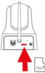
Note: When you plug in the micro SD-card while the camera is powered, please reboot the camera for the micro SD-card to work properly.
