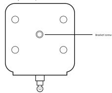
Bracket screw – this is the position to screw in the bracket of the EM6325. With the bracket, you can install the EM6325 on the wall.
