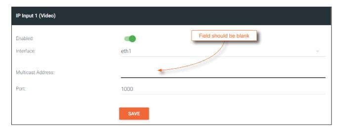
9. Unicast setup is complete. The decoder unit will now receive streams exclusively from the encoder containing the IP address of this decoder.
