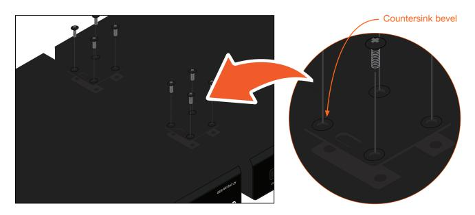
3. Turn the attached units over and install the rack ears (sold separately) to one side of each enclosure using the included screws.
