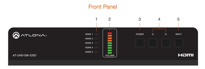
1 HDMI 1 - HDMI 5: Input LED Indicators These LED indicators display which input is routed to the HDMI OUT port. A solid blue indicator represents the active input being used
