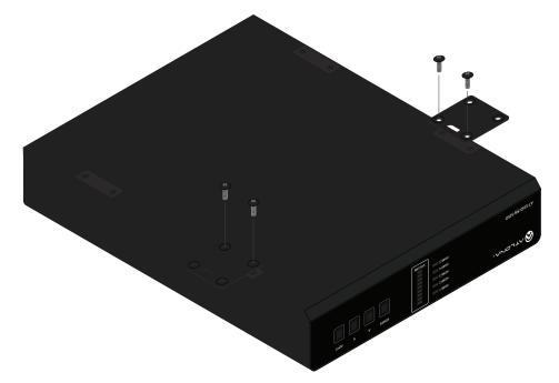
3. Mount the unit using the circular holes, on each mounting plate. If using a drywall surface, a #6 drywall screw is recommended. Mounting screws are not included.
